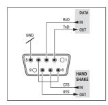
Every balance is equipped with an RS232C interface for connection to a peripheral device (e.g. printer, auxiliary display or PC with a 9-pin male connector, see Section 6.4). The balance must then configured to suit the peripheral device in a menu dialog (Sections 4.3.8 – 4.3.13).
